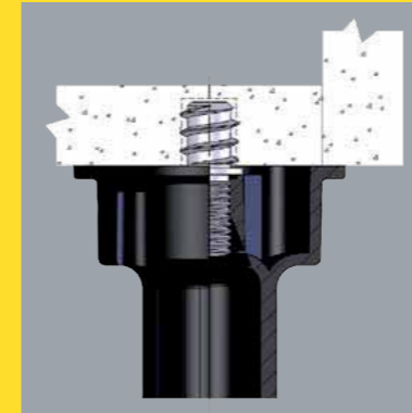
PERNO AUTOFILETTANTE SELF-TAPPING PIN
